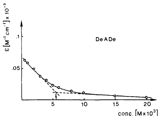
Figure 2. Apparent molar extinction coefficient \epsilon of decylammonium decanoate (DeADe) with AO ( 2 \times 10^{-5} M) in benzene at 25 °C and \lambda 490 nm vs. the concentration of DeADe. Example for the Corrin-Harkins method. 9
